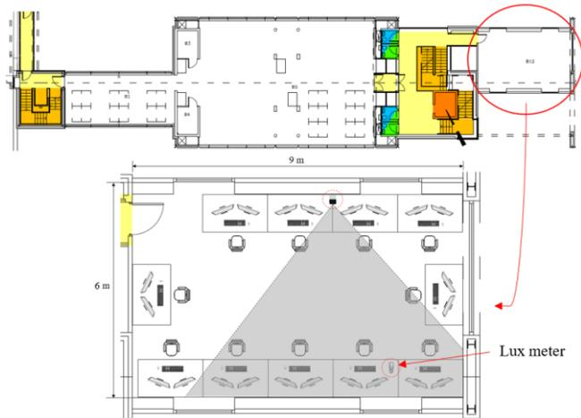
Fig 2 Floor plan and experimental setup of the test room
