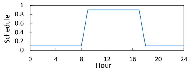
Fig 3 Typical or static daily equipment usage profile
