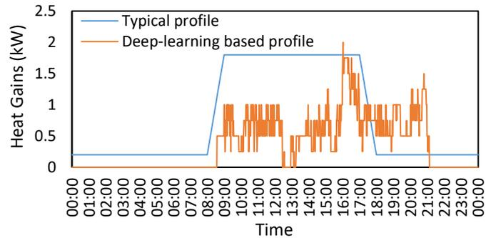
Fig 4 Daily equipment heat load profile
