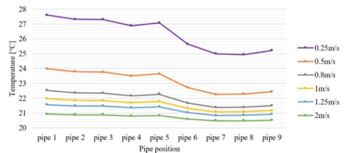
Figure 9. Outlet water temperatures of the nine pipes
