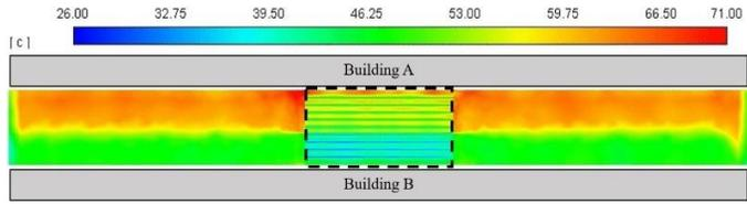
Figure 5. Temperature contour of pavement with PSC with inlet water velocity of 0.25 m/s
