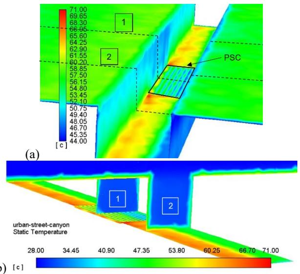
Figure 4. (a) Surface temperature contour of the street canyon and surrounding buildings and (b) cut section temperature contour of the urban street canyon
