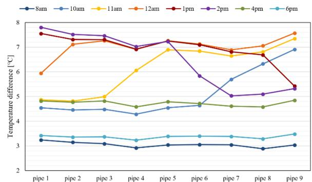
Figure 12. The temperature difference between outlet and inlet water – at different times
