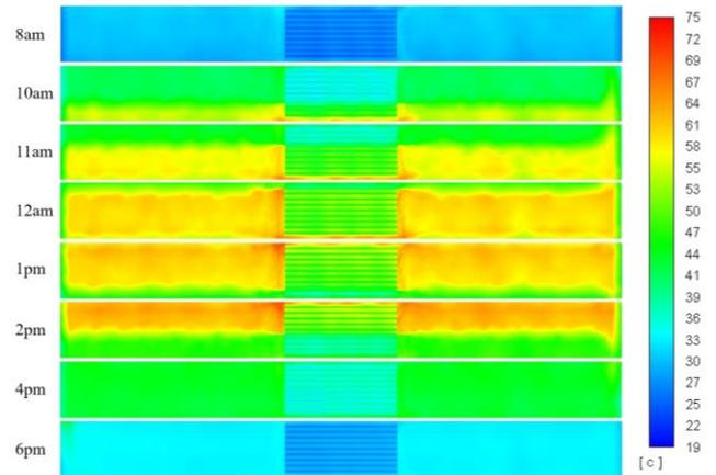
Figure 11. Pavement surface temperature contours at different times
