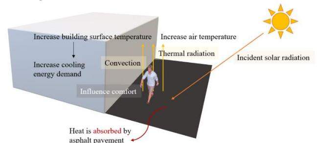
Figure 1. Typical heat transfer in an urban area with a standard pavement [3]
