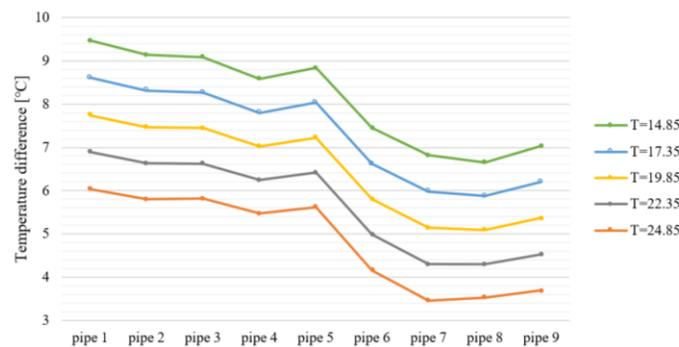
Figure 10. The temperature difference between outlet and inlet water
