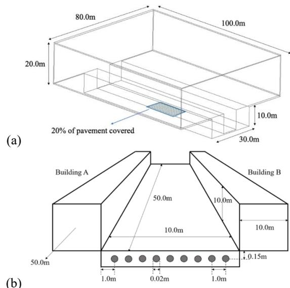
Figure 3. (a) Geometry of the whole domain and (b) location of the pipes (section from Figure 3 (a), not to scale)
