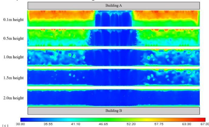
Figure 6. Air temperature distributions in different heights: horizontal cross-section contours from 0.1m to 2m
