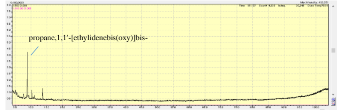
Fig.7 GC-MS chromatogram of collected tar (500ON10)
