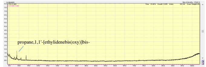
Fig.6 GC-MS chromatogram of collected tar (500OFF)
