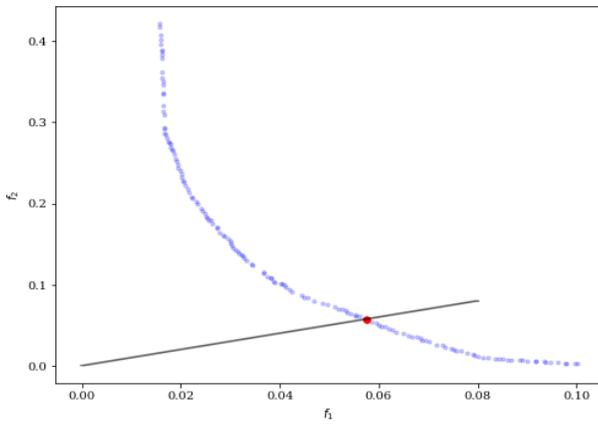
Fig.5. Optimal decomposition point, red dot refers to the compromised solution among two objectives (5%,5%).
