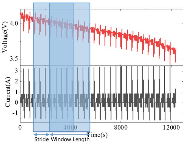
Fig. 2. Data preprocess by moving window
