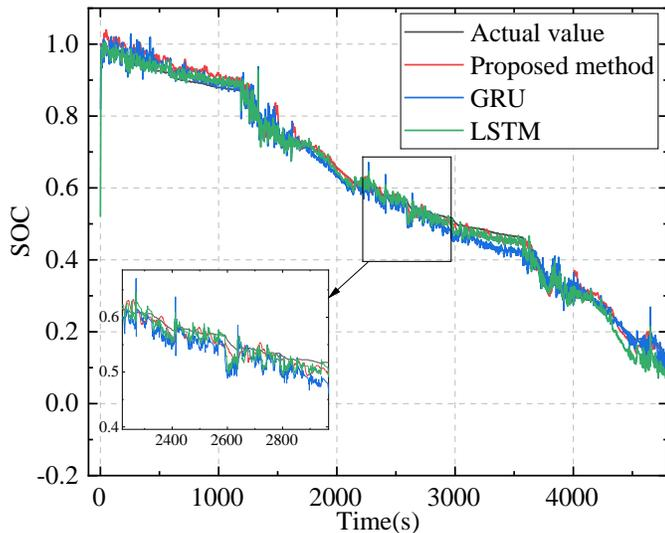
Fig. 6. Results of SOC estimation (Trained by US06 and tested by cycle 4).
