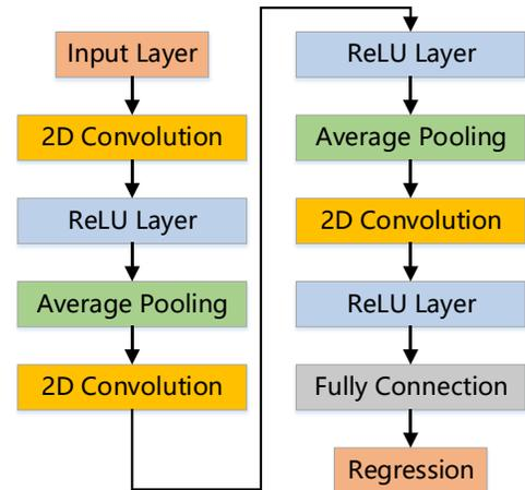
Fig. 3. Structure of proposed DCNN
