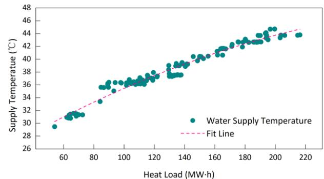
Fig.2 Correlation between water supply temperature and heat load
