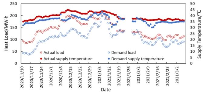
Fig.11 Actual and demand values of heat load and supply temperature
