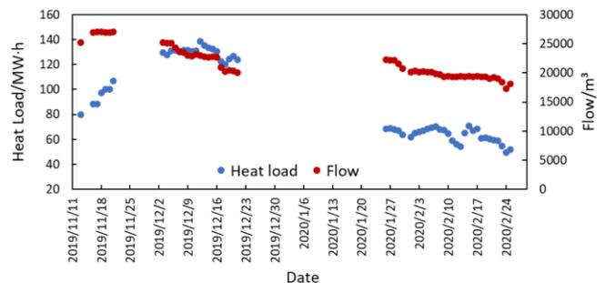
Fig.9 Actual heat load and flow ( 2019-2020 heating season )
