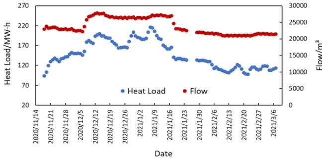
Fig.6 Actual heat load and flow ( 2020-2021 heating season )
