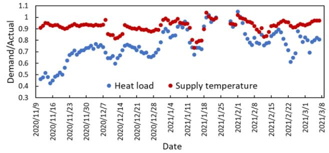
Fig. 12 Ratio of demand load to actual load and demand supply temperature to actual supply temperature ( 2020-2021 heating season )
