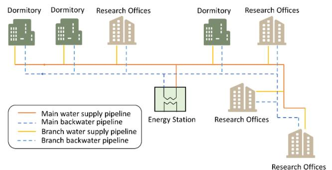
Fig.5 Simplified physical model of the central heating system
