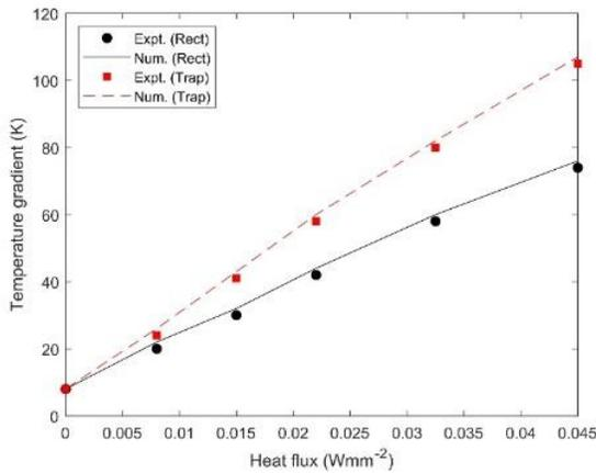
Fig. 2. Validation of TEG's numerical model using experimental data [30]
