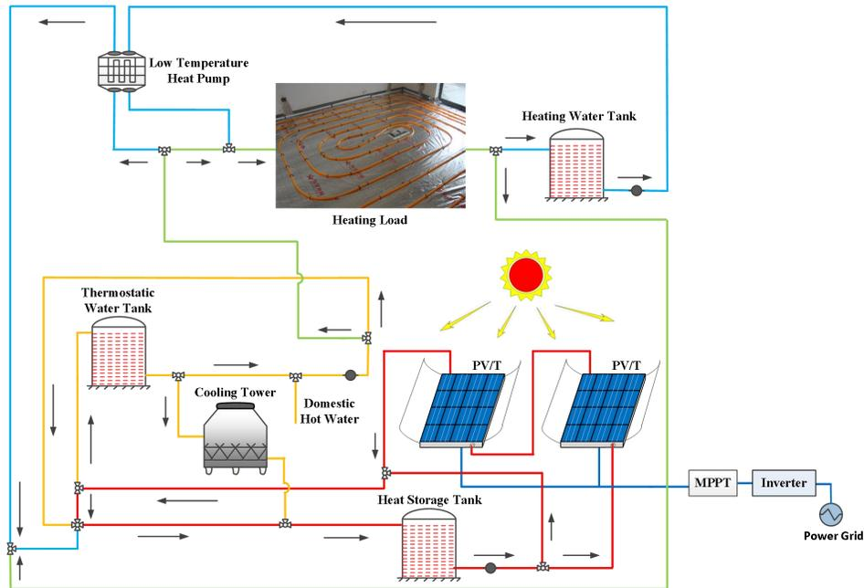
Fig 2 LCPV/T heat pump coupled cogeneration system of villa
