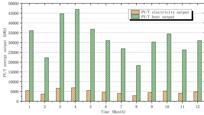
Fig. 4 Monthly power and heat production of LCPV/T system throughout the year
