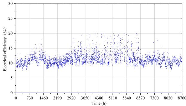
Fig. 5 Annual electric efficiency of LCPV/T system
