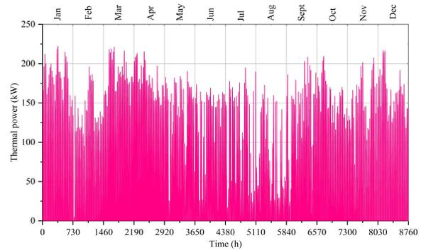
Fig. 3 Annual thermal power of LCPV/T system
