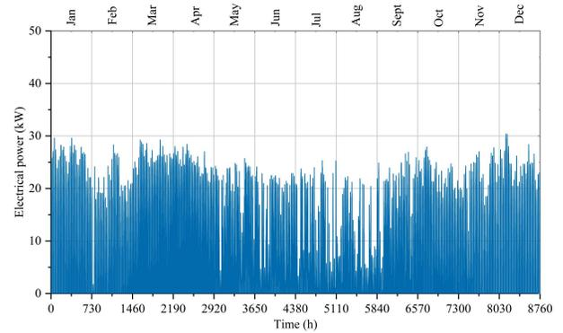
Fig. 2 Annual electric power of LCPV/T system
