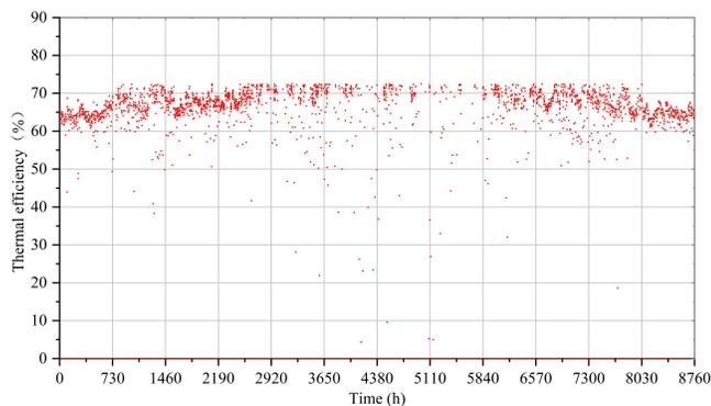
Fig. 6 Annual thermal efficiency of LCPV/T system
