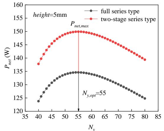
Fig. 6 Change of net power with  $N_y$  at different number of sections
