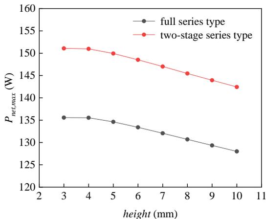
Fig. 8 The optimal net power varies with channel height under different circuit connection modes
