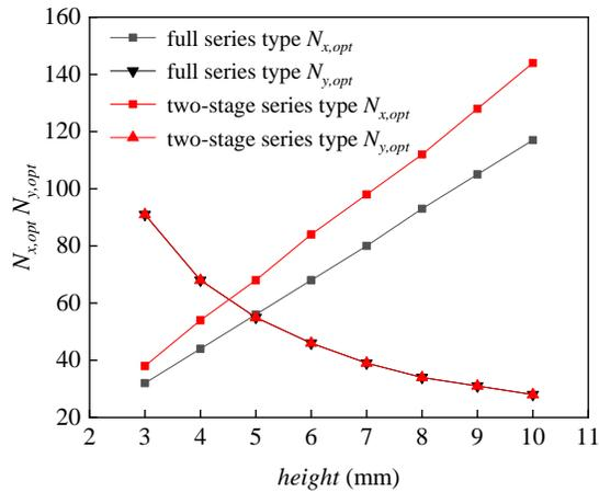
Fig. 7 Optimum length width varies with channel height under different circuit connection modes
