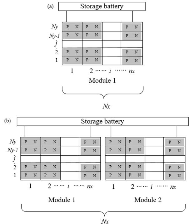
Fig. 2 Schematic diagram of series circuit layout for thermoelectric generator(a) full series type (b) two-stage series type
