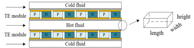
Fig. 1 Overall structure of thermoelectric generator
