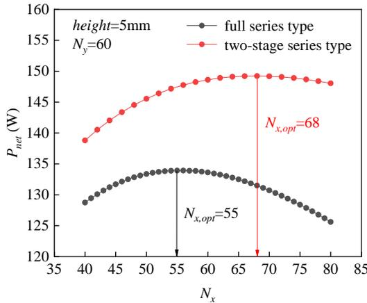
Fig. 4 Variations of net power with  $N_x$  at different number of sections
