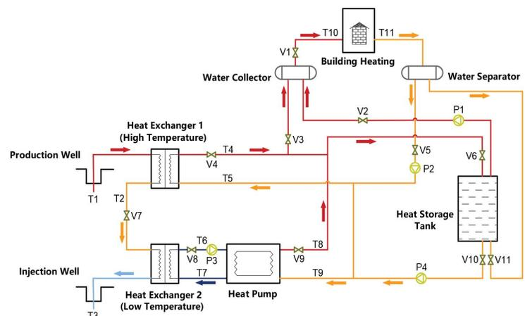
Fig. 1 Energy storage-geothermal coupled heating system
