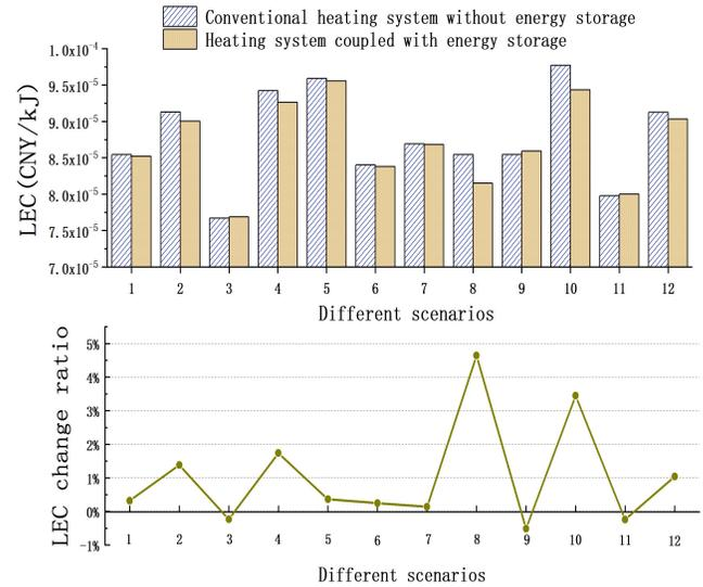
**Fig. 5** Optimal LEC of each scenario – comparison between the conventional heating system and the heating system coupled with energy storage
