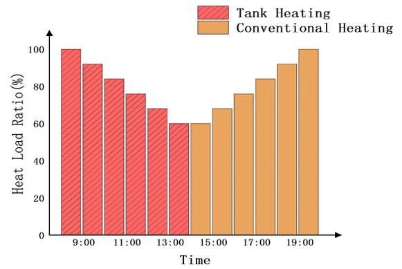
Fig. 2 Daytime heating operation mode
