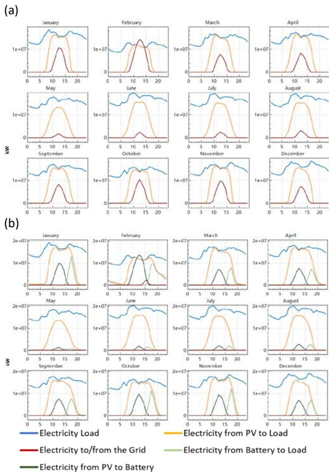
Fig. 4. Comparison of hourly PV generation and destination, EV charge and discharge and load between 2030 PV only (a) and 2030 PV+EV (b) scenarios
