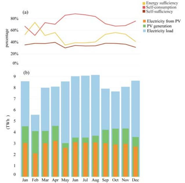
Fig. 3. 2020 monthly key indicators(a) and PV generation, load, and electricity from PV(b)
