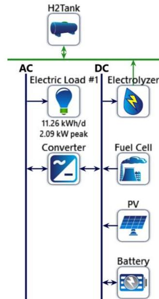
Figure 3. Schematic diagram of system 3 (PV/battery bank/hydrogen).
