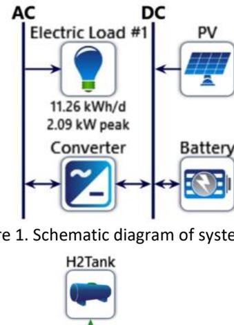
Figure 1. Schematic diagram of system 1 (PV/battery bank).
