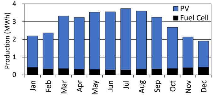
Figure 8. Monthly electric production of system 2.
