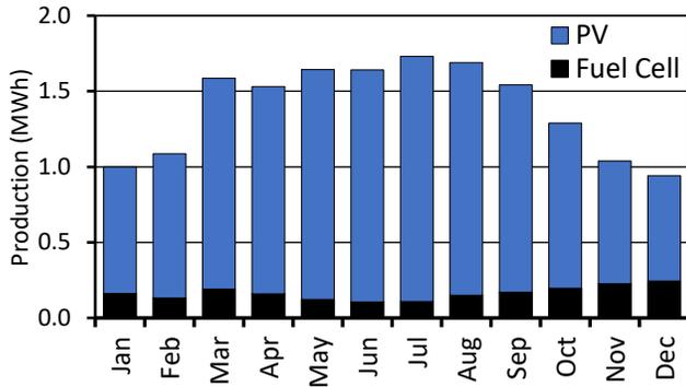
Figure 10. Monthly electric production of system 3.
