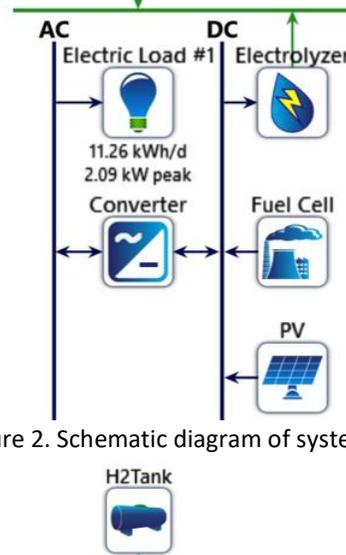
Figure 2. Schematic diagram of system 2 (PV/hydrogen).
