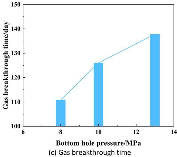
Fig. 3. Development parameters of different bottom hole pressure
