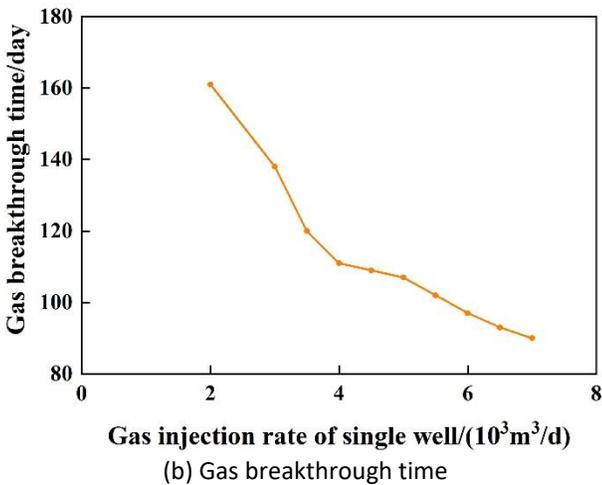
(b) Gas breakthrough time
