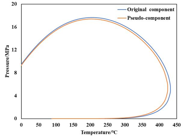
Fig. 1. Phase characteristics fitting diagram of crude oil
