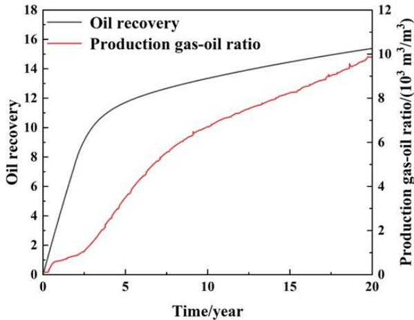
Fig. 5. Oil recovery and production gas-oil ratio for the block
