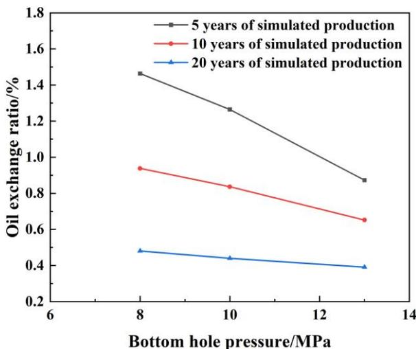
Fig. 4. Oil exchange ratio under different bottom hole pressure
