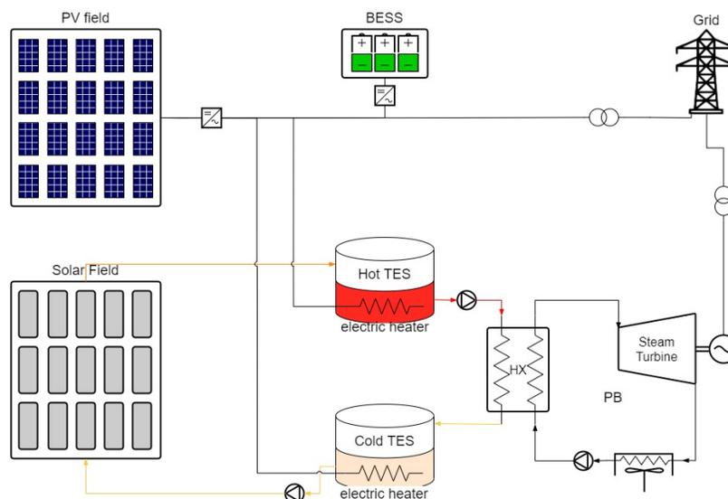
Fig. 1. CSP-PV Hybrid plant scheme
