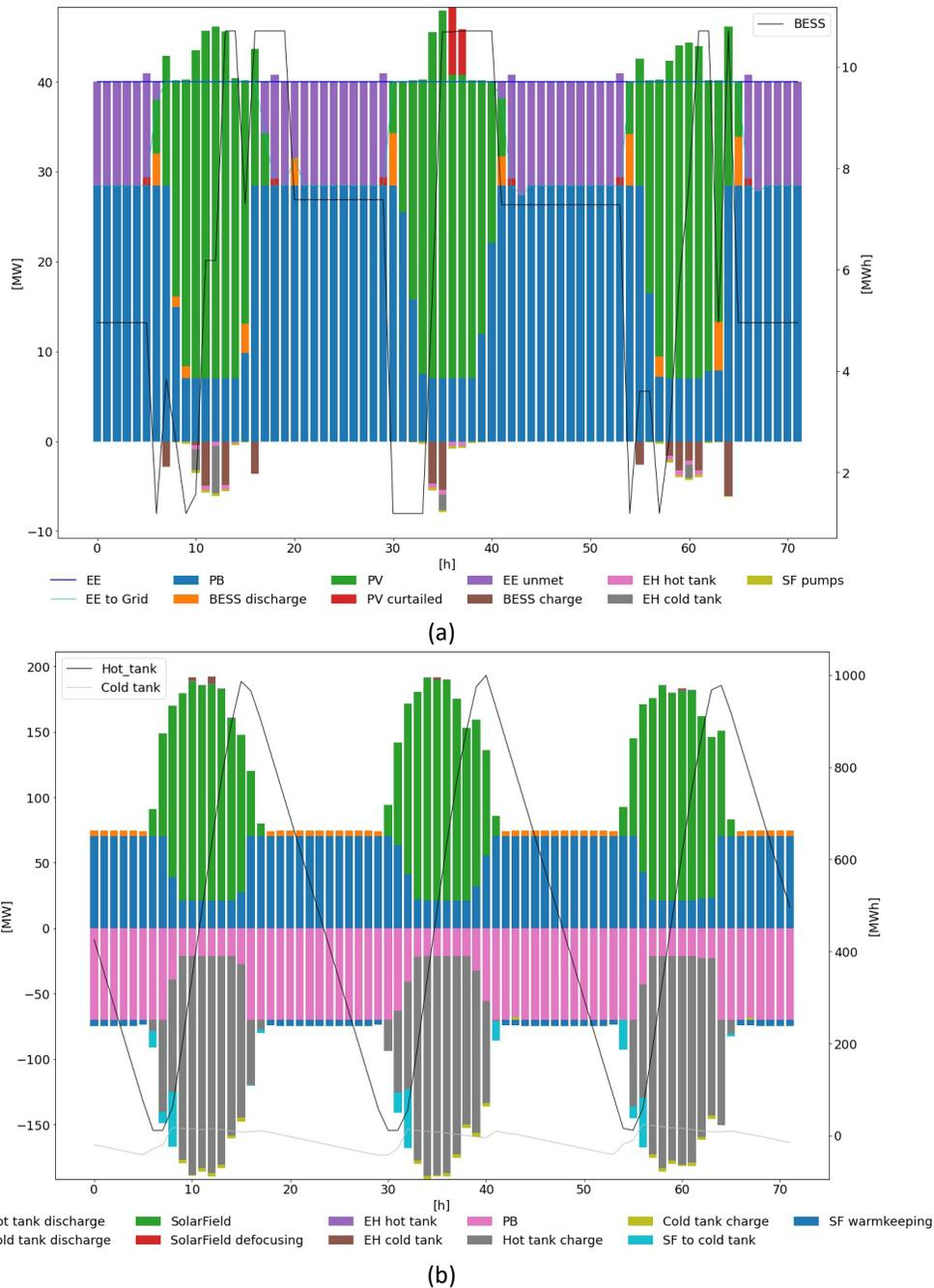
Fig. 2. Electricity (a) and heat (b) balances in a typical period operation characterized by high solar radiation.
