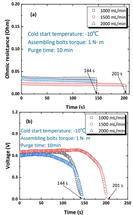
Fig. 7 The effect of purge gas flow on cold start: (a) ohmic resistance change and (b) voltage change
