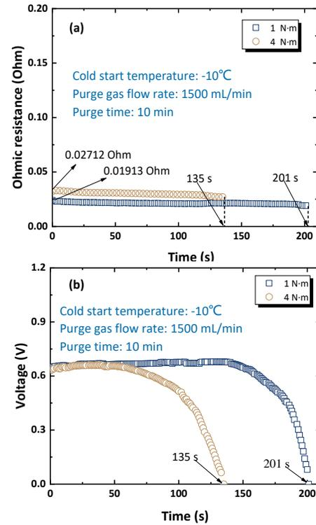
Fig. 4 Effect of assembling bolt torque on cold start: (a) ohmic resistance change and (b) voltage change
