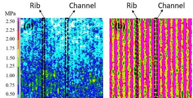
Fig. 3 Pressure distribution between CL and MPL: (a) 1 N·m and (b) 4 N·m
