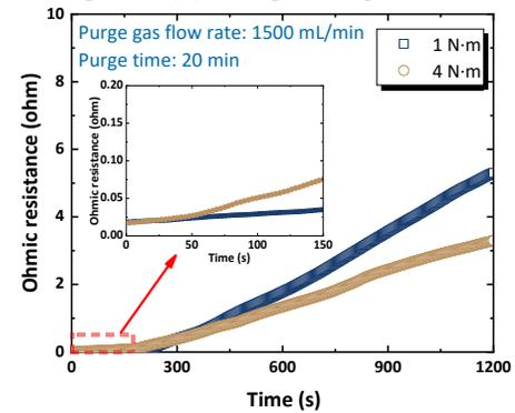
Fig. 5 Ohmic resistance change during purge process
