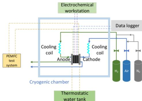
Fig. 2 Schematic diagram of PEMFC purge and cold start experimental system
