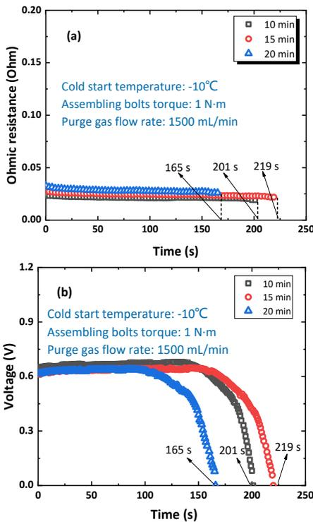
Fig. 6 The effect of purge time on cold start: (a) ohmic resistance change and (b) voltage change
