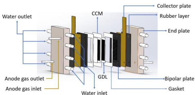
Fig. 1 Schematic diagram of fuel cell structure
