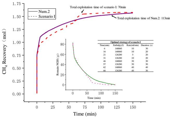
Figure 3. CH<sub>4</sub> recovery curve of scenario I compared with the control group.
