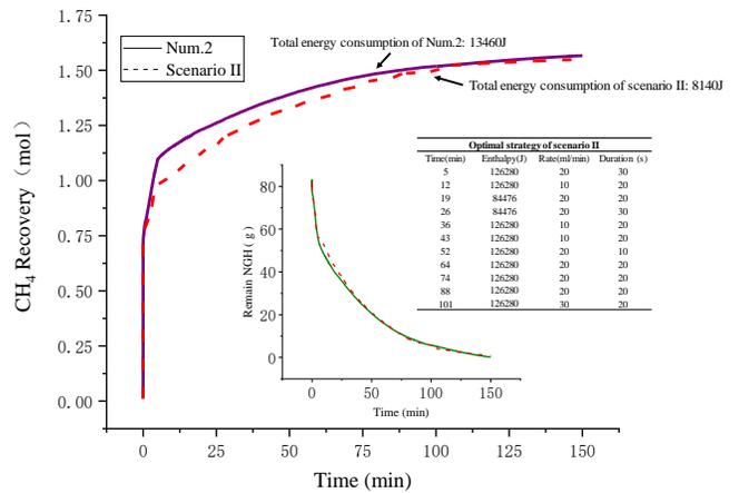
Figure 4. CH<sub>4</sub> recovery curve of scenario II compared with the control group.
