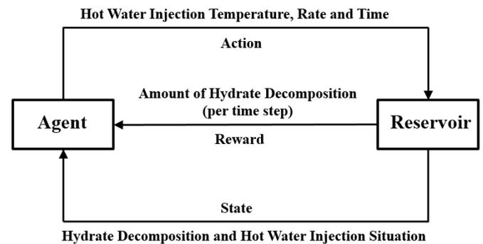
Figure 1. Schematic diagram of interaction between agent and deposits
