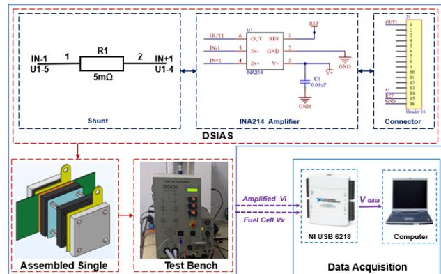
Fig 2 DSIAS test schematic
