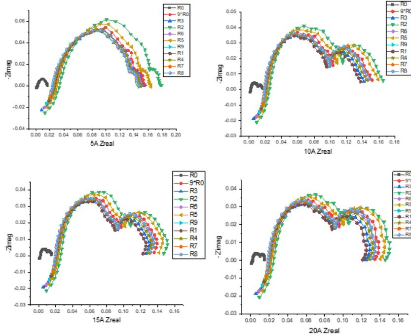
Fig 3 The cell single and segments impedance spectrum
