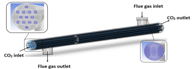
Fig. 2. The physical and mesh model of the simulated shell-and-tube heat exchanger
