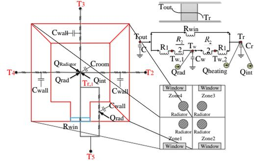
Fig. 2. RC model of one heating zone
