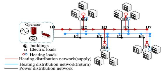
Fig. 3. Schematic of the electricity and heating distribution networks of the system
