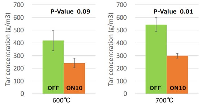
Fig.6 Tar concentration in the syngas (Polypropylene)
