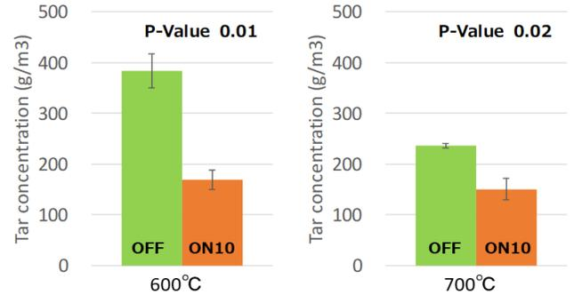
Fig.5 Tar concentration in the syngas (cellulose)
