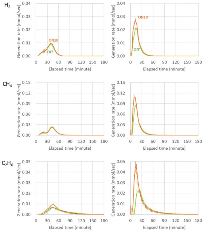
Fig.4 Generation rate of H<sub>2</sub>, CH<sub>4</sub>, C<sub>2</sub>H<sub>6</sub> (Polypropylene)
