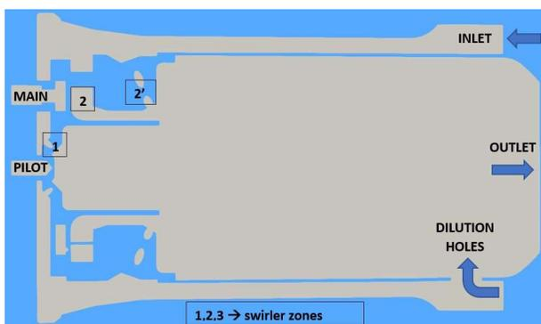
**Figure 1.** Schematic cross section of T100 combustor, highlighting the counter-flow air inlet on the outside of the chamber, as well as the pilot (1) and main (2) flame injectors, as well as the dilution holes.
