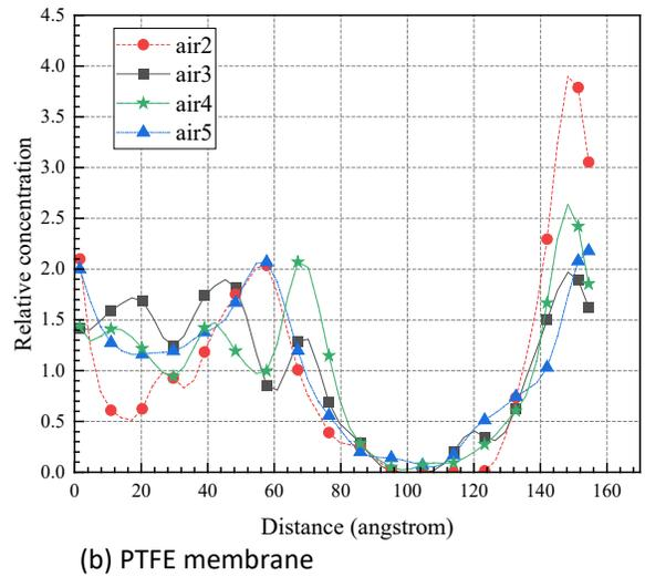
Fig. 4. Relative concentration of CO<sub>2</sub> in the layers
