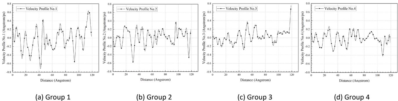
Fig. 5. Average velocity profile along the z-axis of CO<sub>2</sub> molecules in 500 ps
