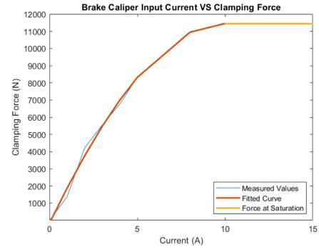
Fig. 3. Brake Caliper Input Current VS Clamping Force
