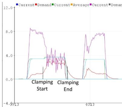
Fig. 8 One Actuation-Retracton Cycle, With Pedal, Current and Motor Speed Values
