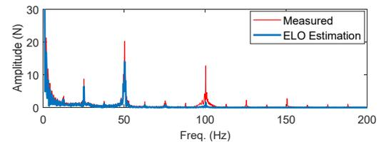
Fig. 7 The Frequency spectrum of the measure force and estimated one by the ELO.
