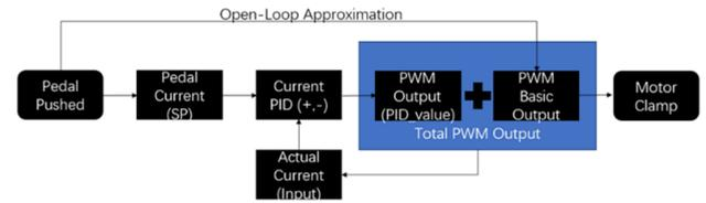
Fig. 4. The Algorithm of Closed-loop Current Control
