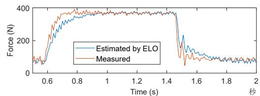
Fig. 6 The clamping force estimation in the regular braking mode: the measured force versus the estimated force by the ELO.
