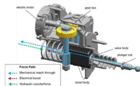
Fig. 1. An Electro-Mechanical Brake Booster
