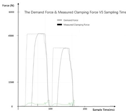
Fig. 9 Clamp-force control without force sensor
