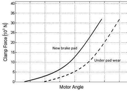
Fig. 2. Characteristic curves of a proposed EMB caliper [5]
