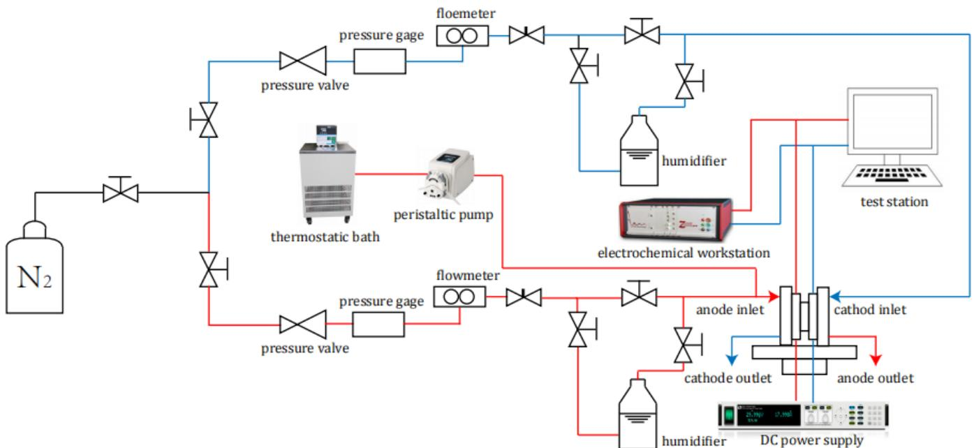
Fig. 2. Schematic diagram of PEMWE test system
