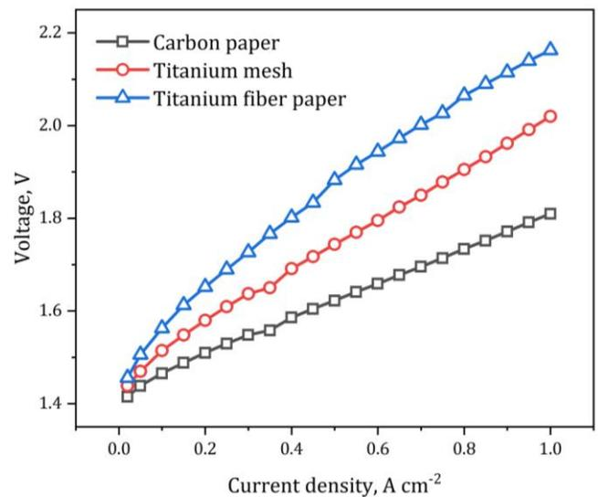
Fig. 5. Polarization curves of PEMWE with different LGDLs
