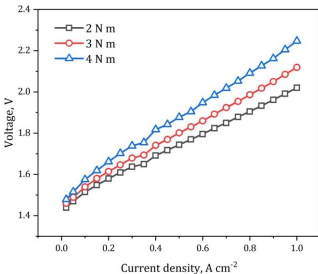
Fig. 4. Comparison of titanium mesh as anode LGDL under different torques (2 N m, 3 N m and 4 N m)
