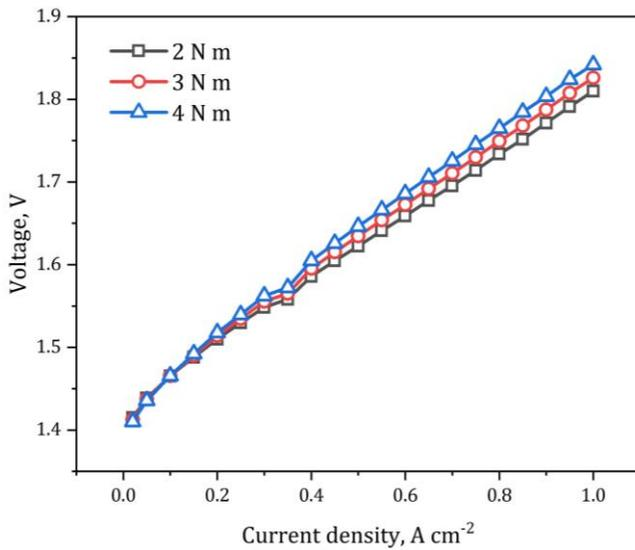
Fig. 3. Comparison of carbon paper as anode LGDL under different torques (2 N m, 3 N m and 4 N m)
