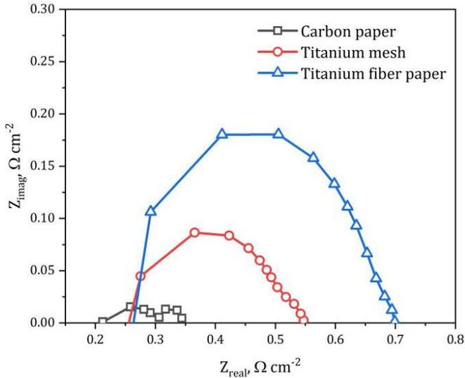
Fig. 6. Electrochemical impedance spectroscopy of PEMWE with different LGDL
