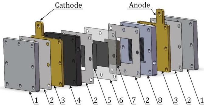
Fig. 1. Schematic diagram of PEMWE
