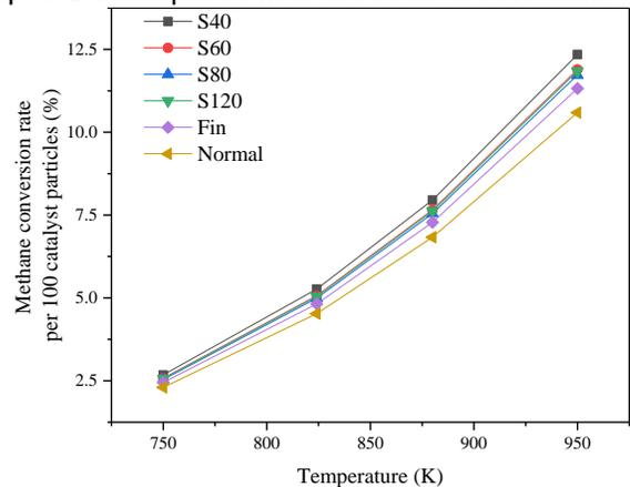
**Fig. 5.** Methane conversion rate per 100 catalyst particles for different temperature
