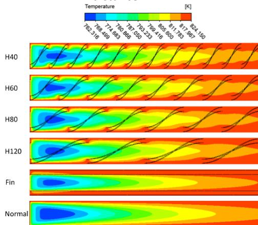
Fig. 7. Temperature contour in Longitudinal section of different structures
