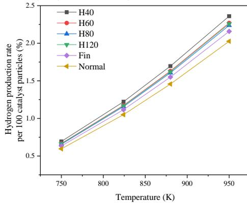
Fig. 6. Hydrogen production rate per 100 catalyst particles for different temperature
