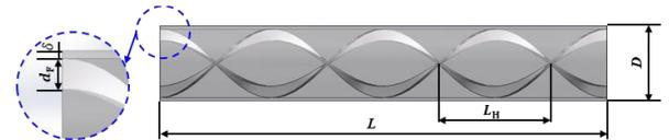
Fig. 2. Detailed information for internal spiral finned tube
