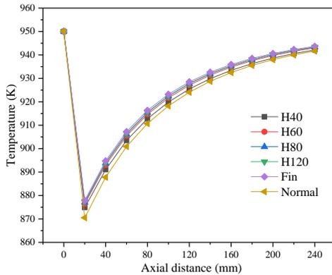
Fig. 7. Average temperature of cross section along axial distance
