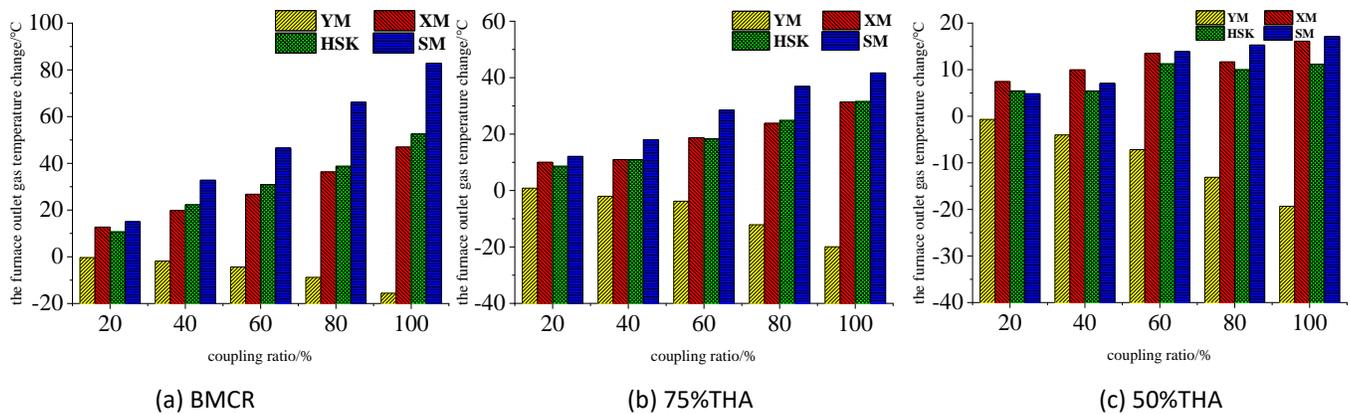
Fig. 2. The effect to the furnace outlet flue gas temperature of biomass blending
