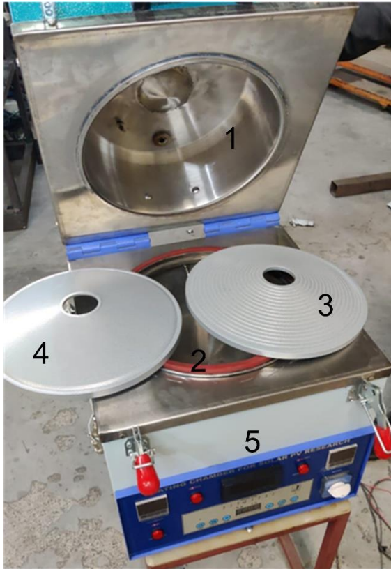
Fig.7. Proposed design of system (1) Condensing chamber (2) Evaporating Chamber (3) Upper heat sink of TEM (4) Lower heat sink of TEM (5) Controller of heating element
