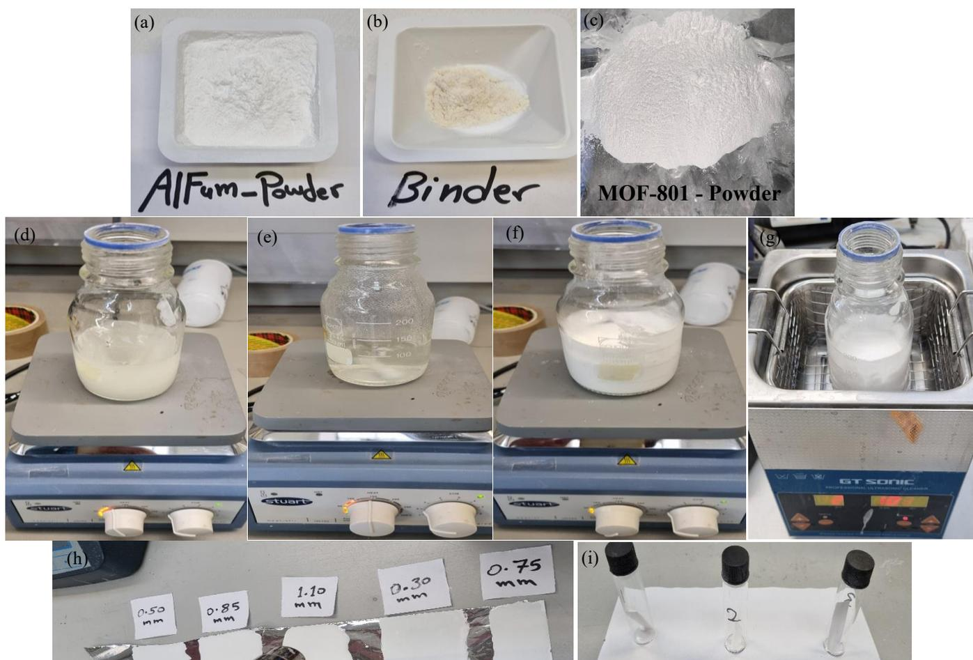
Figure 1. Optical images for MOFs coating synthesis. (a) AlFum-powder, (b) binder, (c) MOF-801 – powder, (d, e) binder solution preparation, (f, g) MOF/binder solution preparation, (h) dip coating MOFs on aluminum foil with different thicknesses and (i) MOFs different thicknesses ready for characterizations after drying
