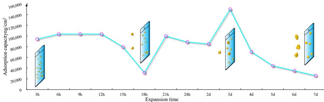
Fig 4 Cumulative adsorption of HPAM nanoparticles
