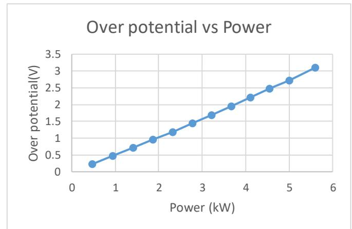
Fig. 3. Plot against over potential and power deduced from polarization plot.
