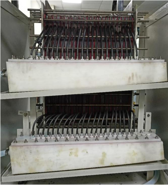
Fig.1. 5 kW VRFB stack with 22 cells of 1500 cm<sup>2</sup> active area and external manifolds for electrolyte circulation.
