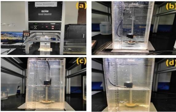
Fig. 1. Experimental setup (a) Solar simulator and submerged pyranometer; submerged pyranometer in (b) DDW, (c) LTLW and (d) HTLW
