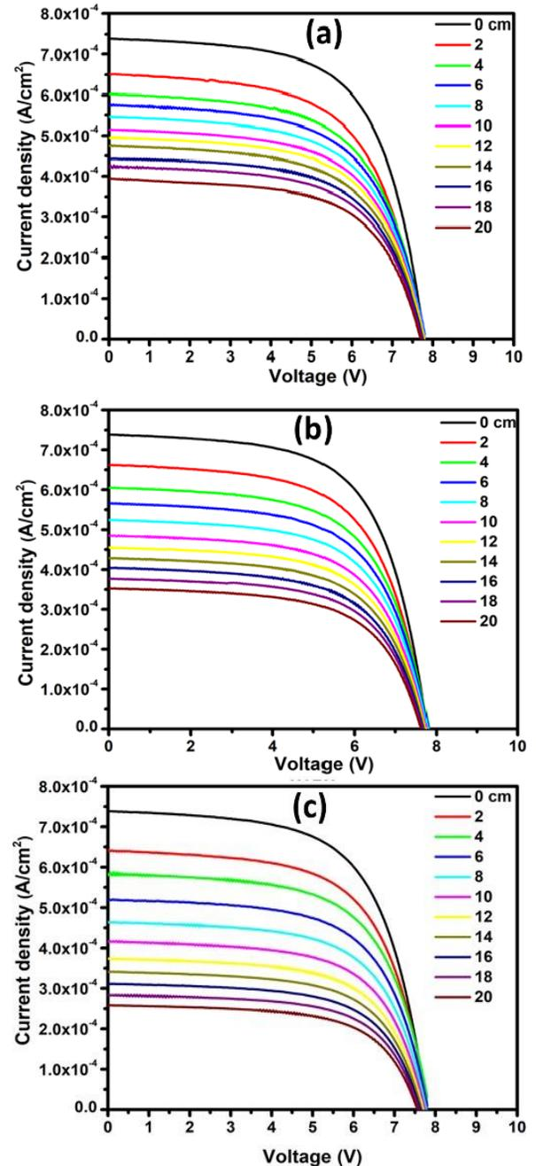
Fig. 3. J-V characteristics for a-Si solar cell with respect to depth for (a) DDW, (b) LTLW and (c) HTLW
