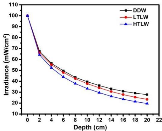
Fig. 2. Variation of irradiance power with the increasing depth in DDW, LTLW and HTLW
