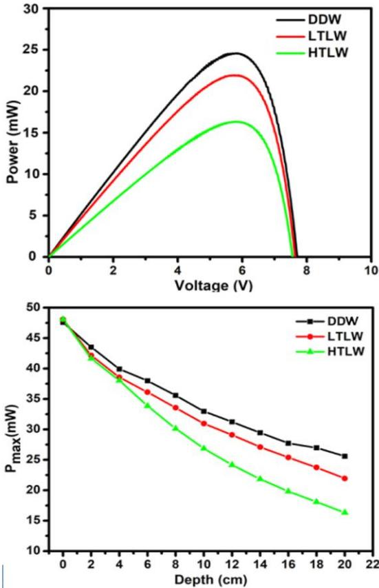
Fig. 4. (a) Variation of power with voltage in different water environments at 20 cm and (b) Variation of  $P_{max}$  values at different depths for all the water environments
