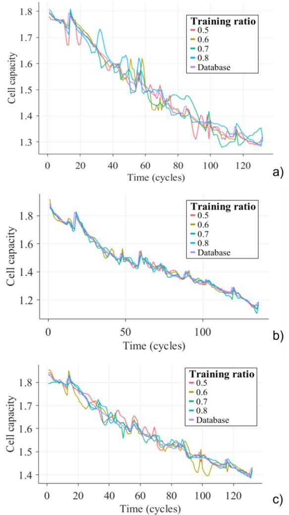
Fig. 6. The DCNN learning result for battery SOH estimation for B0007 validation dataset
