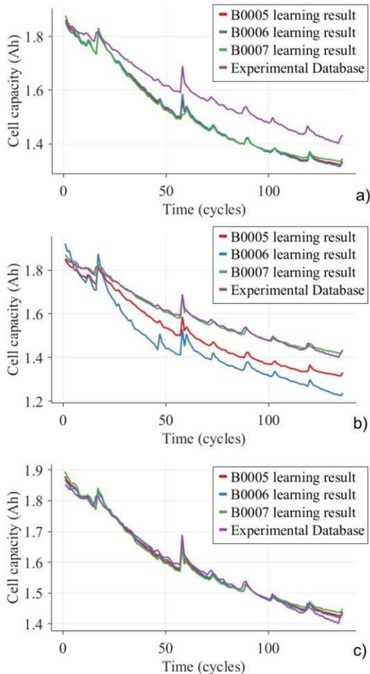
Fig. 7. The DCNN learning result for battery SOH estimation for B0006 validation dataset
