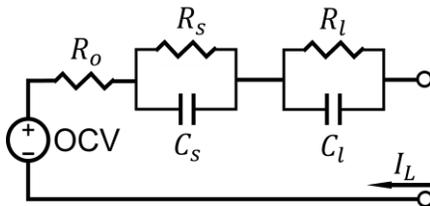
Fig. 1. The second order RC equivalent circle model
