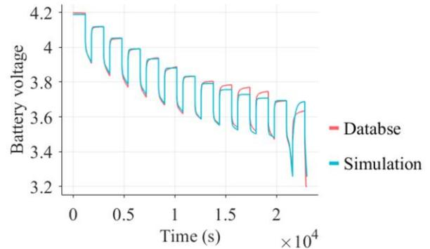
Fig. 5. Performance of voltage comparison for battery modelling
