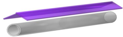
(a) Structure of secondary reflector
