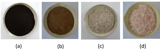
Fig. 1 Materials used are (a) low-rank coal (b) EFB (c) PET bottle waste (d) plastic bag waste
