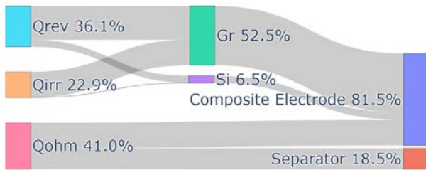
Fig. 5 Sankey chart for percentage contribution of heat sources when mr = 0.1 electrodes at a galvanostatic 2C delithiation condition.
