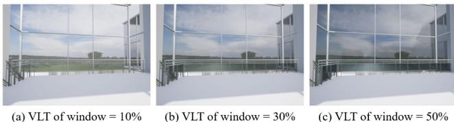
Fig. 1 Virtual environments according to the different VLT of window-integrated PV panels
