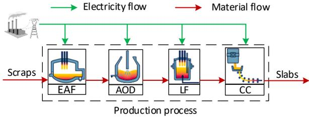
Fig. 1 The Scheme of Steel Production Process
