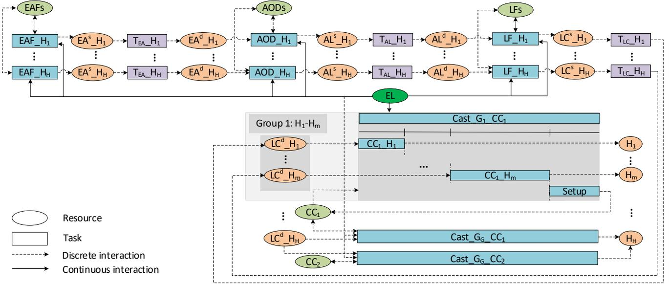
Fig. 2 Resource Task Network for Production Scheduling of a Steel Plant
