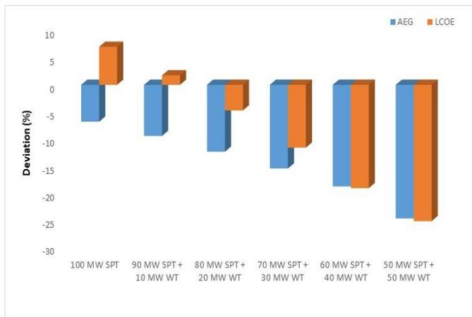
**Fig. 3.** Evolution of the AEG and LCOE for different SPT-WT combinations of 100 MW capacity.
