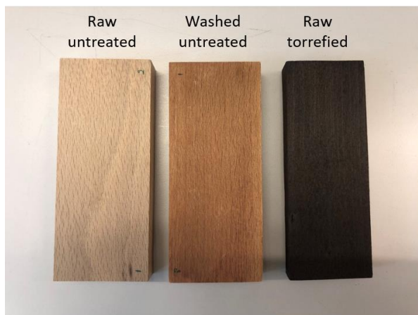
Fig. 3 Color change of wood blocks with impregnation and torrefaction
