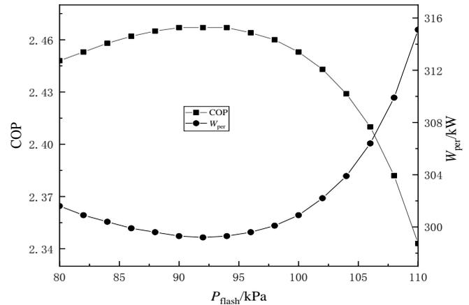
Fig.5 The COP and  $W_{per}$  vs.  $P_{flash}$  of the CF-SGHP system
