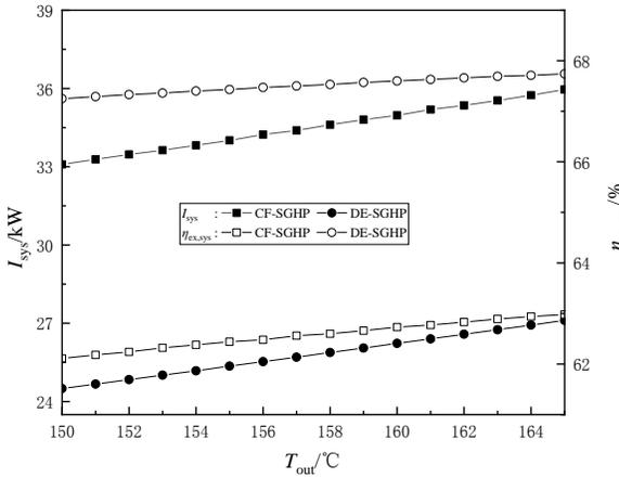
Fig.8.  $I_{sys}$  and  $\eta_{ex,sys}$  vs.  $T_{out}$  of the heat pump steam systems
