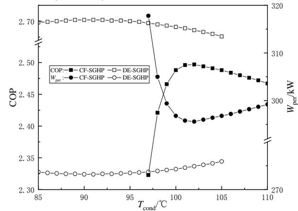
Fig.11. COP and  $W_{per}$  vs.  $T_{cond}$  of the heat pump steam systems
