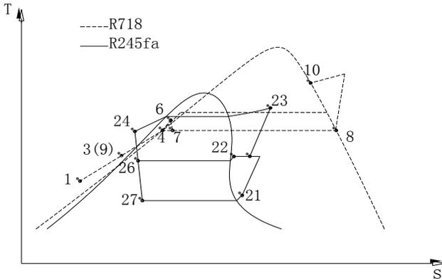
Fig.2. T-S diagram of the refrigerants in the CF-SGHP system
