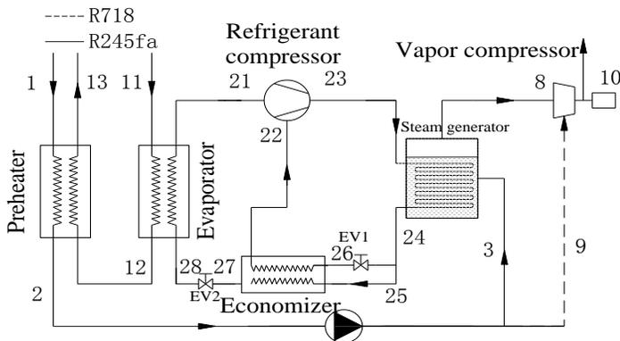
Fig.6. Flowsheet of a direct evaporative heat pump generator steam system
