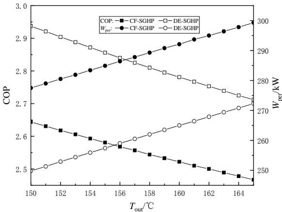
Fig.9. COP and  $W_{per}$  vs.  $T_{out}$  of the heat pump steam systems
