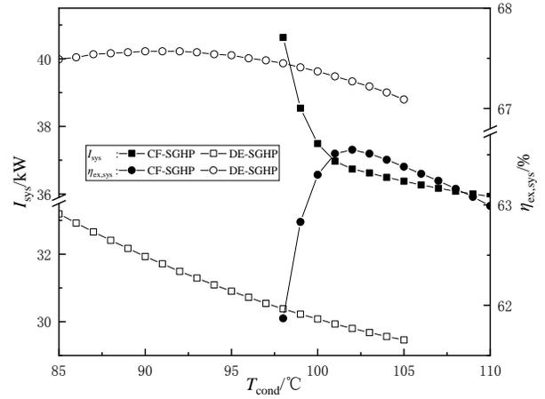
Fig.10.  $I_{sys}$  and  $\eta_{ex,sys}$  vs.  $T_{cond}$  of the heat pump steam systems
