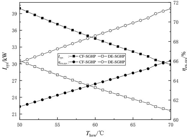
Fig.12.  $I_{sys}$  and  $\eta_{ex,sys}$  vs.  $T_{hsw}$  of the heat pump steam systems
