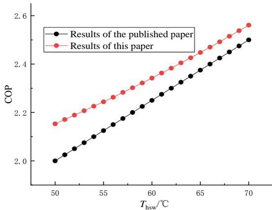
Fig.4 Result of the COP vs.  $T_{hsw}$  calculated by paper's model compared with the published literature
