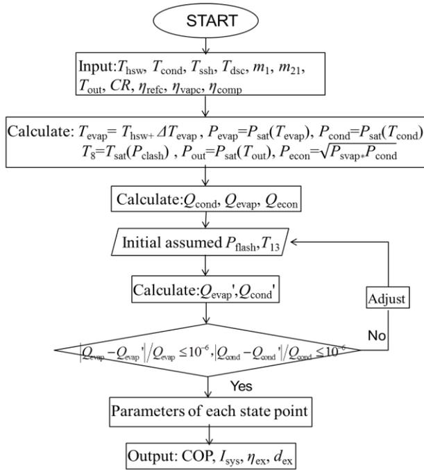
Fig.3. Calculation flow chart of the mathematical model
