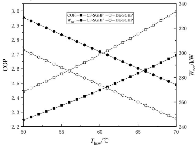
Fig.13. COP and  $W_{per}$  vs.  $T_{hsw}$  of the heat pump steam systems
