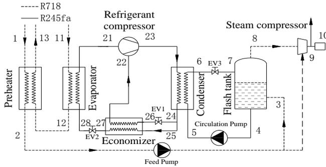
Fig.1. Flowsheet of the circulating flash heat pump steam generator system
