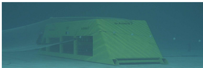
Fig. 5 Trawl net impacting a subsea structure, scaled laboratory test performed at SINTEF Energy Trondheim [11]
