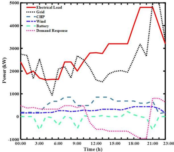
Fig. 5. Electricity Demand Fulfillment Distribution Based on Dynamic Transformer Efficiency
