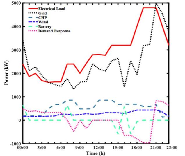
Fig.4. Electricity Demand Fulfillment Distribution Based on Static Transformer Efficiency
