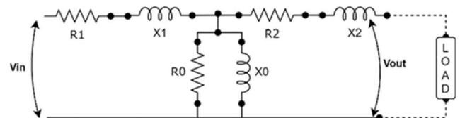
Fig.1. Basic Equivalent Circuit of A Transformer
