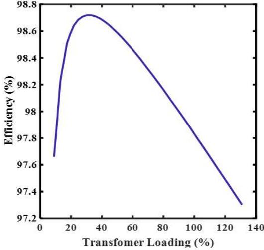
Fig.2. Transformer Efficiency and Loading Percentage
