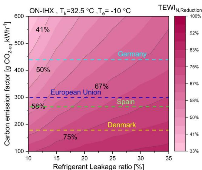
Fig. 7 TEWI<sub>N</sub> Reduction Using R516A
