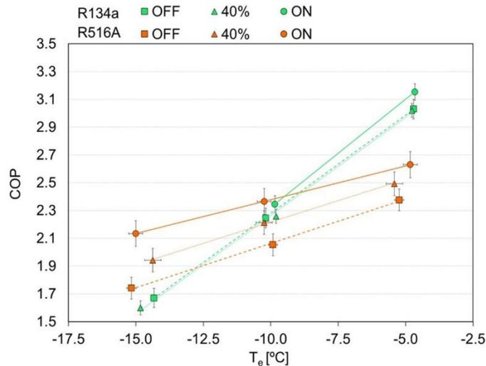
Fig. 6 COP Measurements
