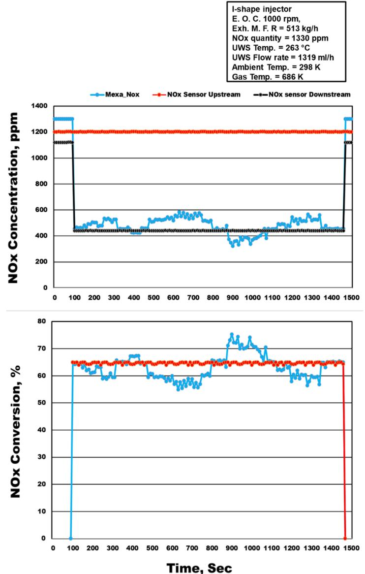
Fig. 4. NOx conversion from L-type Injector in 1000rpm engine operation.
