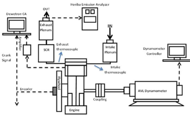
Fig. 3. Schematic diagram of the test engine and measurement setup [7]
