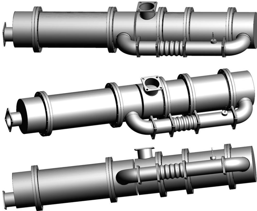
*Fig. 1. The CFD simulation geometry model of the commercial SCR system by HYUNDAI D6CC*
