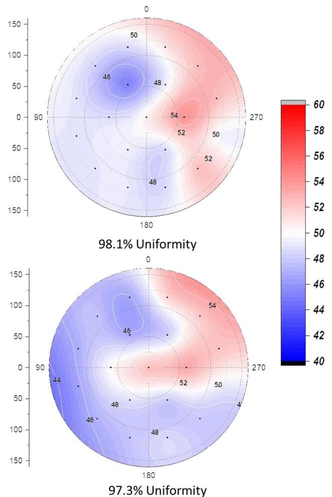
Fig. 6. Ammonia Uniformity from I-type of urea injector and L-type of urea injector.
