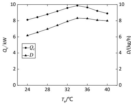
Fig. 3. Influence of outdoor air temperature on system cooling and dehumidification capacity
