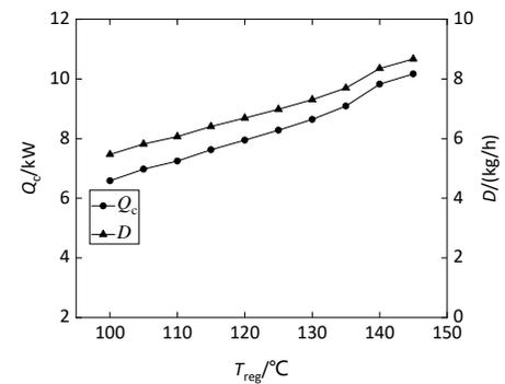
Fig. 7. Influence of regeneration temperature on system cooling and dehumidification capacity
