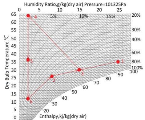
Fig. 2. Psychrometric chart of air treatment process
