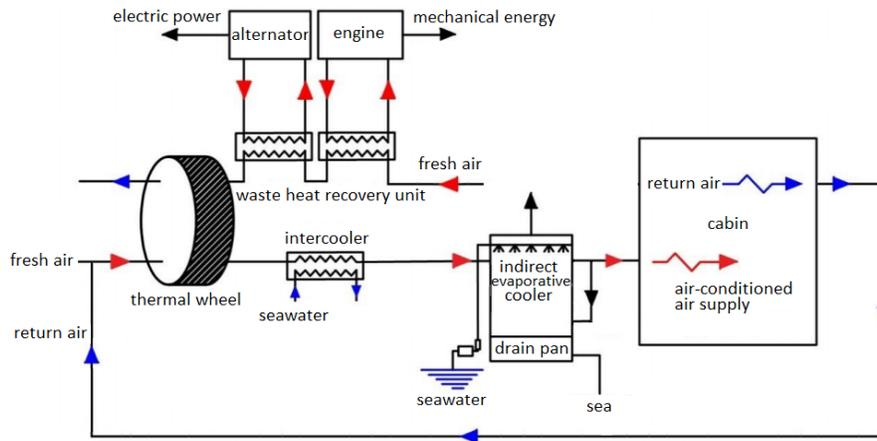
Fig. 1. Schematic diagram of hybrid thermal wheel and evaporative cooling air-conditioning system for marine ships
