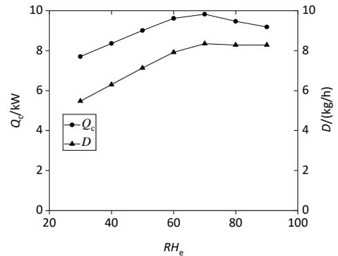
Fig. 5. Influence of outdoor air relative humidity on system cooling capacity and dehumidification capacity
