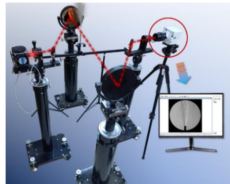
Fig. 1. Visual imaging system for hydrogen leakage.
