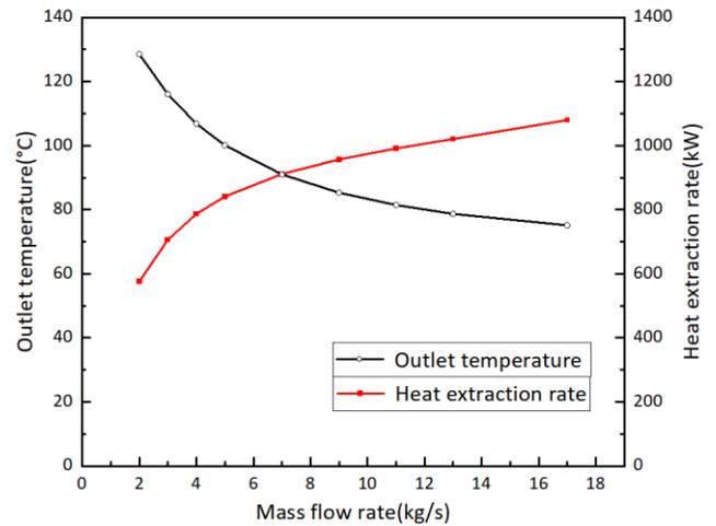
Fig. 6. Outlet temperature and heat extraction rate variations of vertical well with mass flow rate
