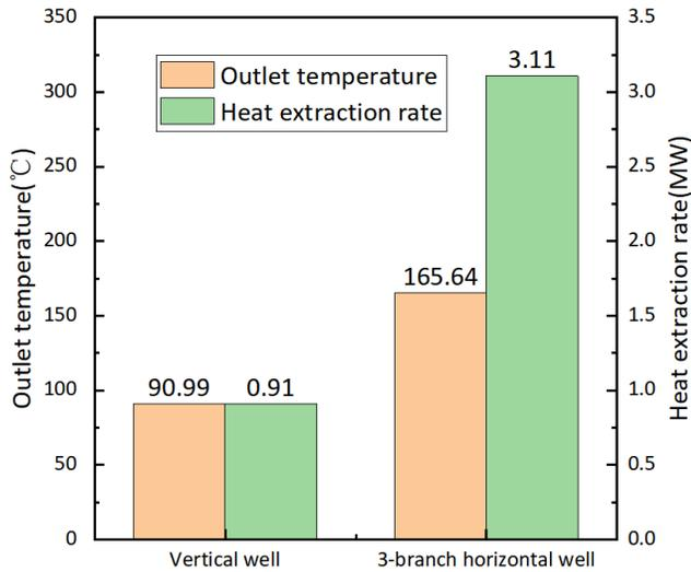
Fig. 7. Outlet temperature and heat extraction rate of vertical well and horizontal well at the end of 120 days
