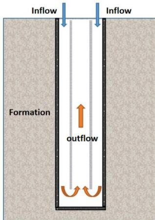
Fig. 2. Closed-loop heat extraction model
