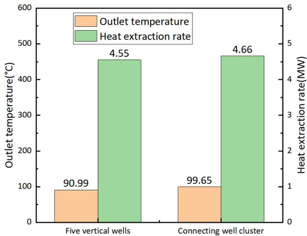
Fig. 8. Outlet temperature and heat extraction rate of vertical well and connecting well cluster at the end of 120 days
