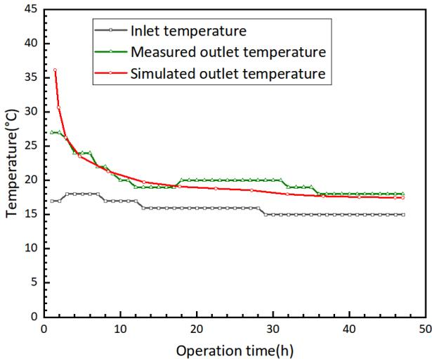
Fig. 5. Fitting curve between measured outlet temperature and simulated outlet temperature
