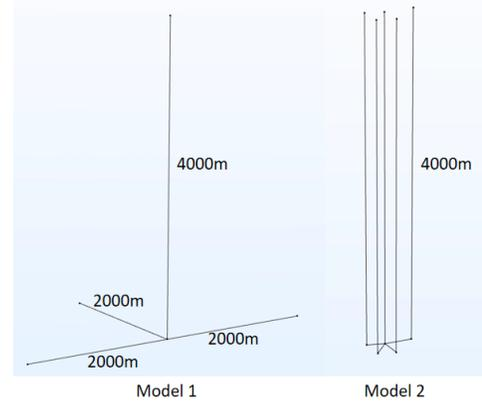
Fig. 3. Schematic diagram of two new geothermal well models
