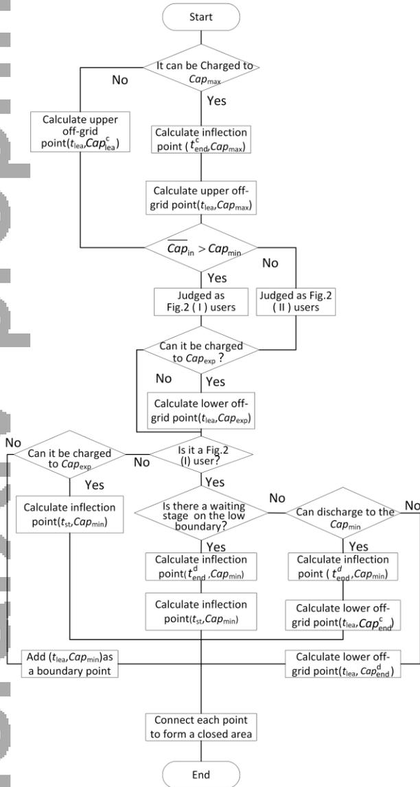
Fig. 3. EV flexibility controllable region construction process
