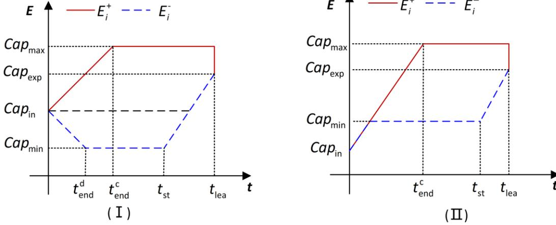
Fig. 2. EV flexibility controllable region under ideal conditions
