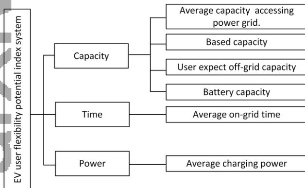
Fig. 1. Flexibility index system of EVs
