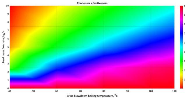
Figure 5. Relationship between boiling temperature, mass flow rate with condenser effectiveness.
