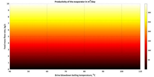
Figure 2. Effect of the brine blowdown temperature and feed mass flow rate on single-effect evaporator productivity.
