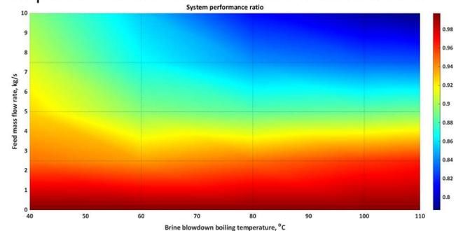
Figure 3. Effect of the brine blowdown boiling temperature and feed mass flow rate on the performance of a single-effect evaporator.
