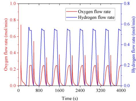
Fig. 4 The outlet hydrogen and oxygen molar flow rates of the STC-SOEC system
