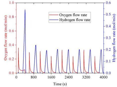
Fig. 3 The outlet hydrogen and oxygen flow rates from the solar reactor
