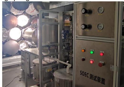
Fig. 1 The photo of the concentrated solar SOEC system
