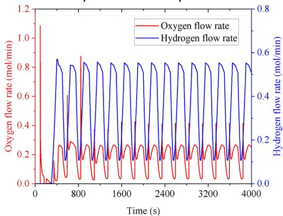
Fig. 5 The outlet hydrogen and oxygen molar flow rates of the DSTC-SOEC system
