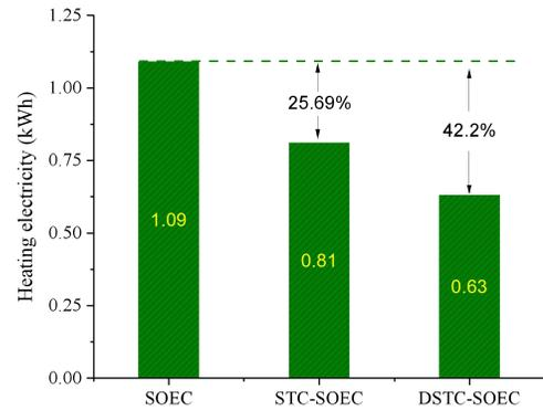
Fig. 6 The comparison of heating electricity among different systems
