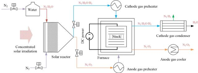
Fig. 2 The combined STC-SOEC system diagram
